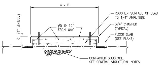
NOTE: LOCATION, SIZE OF PAD (A, B & C DIMENSIONS) AND ANCHOR RODS AS REQUIRED BY EQUIPMENT MANUFACTURER. DRILLED IN EPOXY ANCHORS MAY BE SUBSTITUTED AT CONTRACTOR'S OPTION. (ANCHOR RODS TO BE SUPPLIED BY MISCELLANEOUS METAL SUB-CONTRACTOR AND INSTALLED BY CONCRETE CONTRACTOR)
