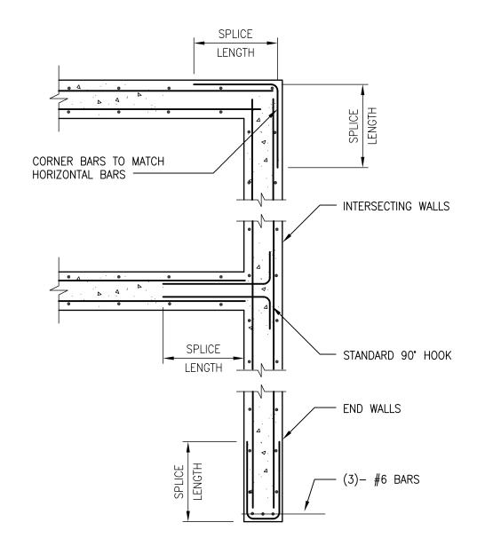
CONCRETE WALL REINFORCING DETAIL SCALE: NONE
